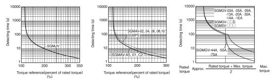
Note: Overload characteristics shown above do not guarantee continuous duty of 100% or more output. Use a servomotor with effective torque within the continuous duty zone of Torque-Motor Speed Characteristics.
